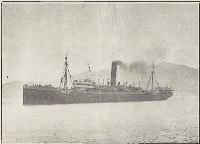
Completed at Belfast, August, 1910, by Messrs. Harland & Wolff, for Shaw, Saville, & Albion Co., Ltd., 10,000 tons. length 477 feet. breadth 63 feet, COMMANDER: R. S. LEWIS.
